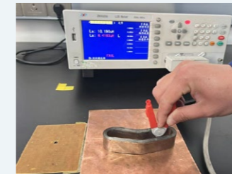
10kHz 0.3V L=10.1μH 100kHz 0.3V L=8.4μH
