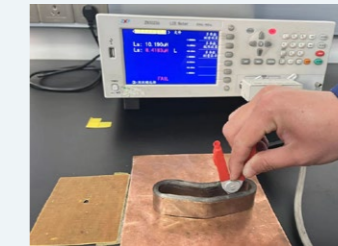
10kHz 0.3V L=10.3μH 100kHz 0.3V L=8.6μH
